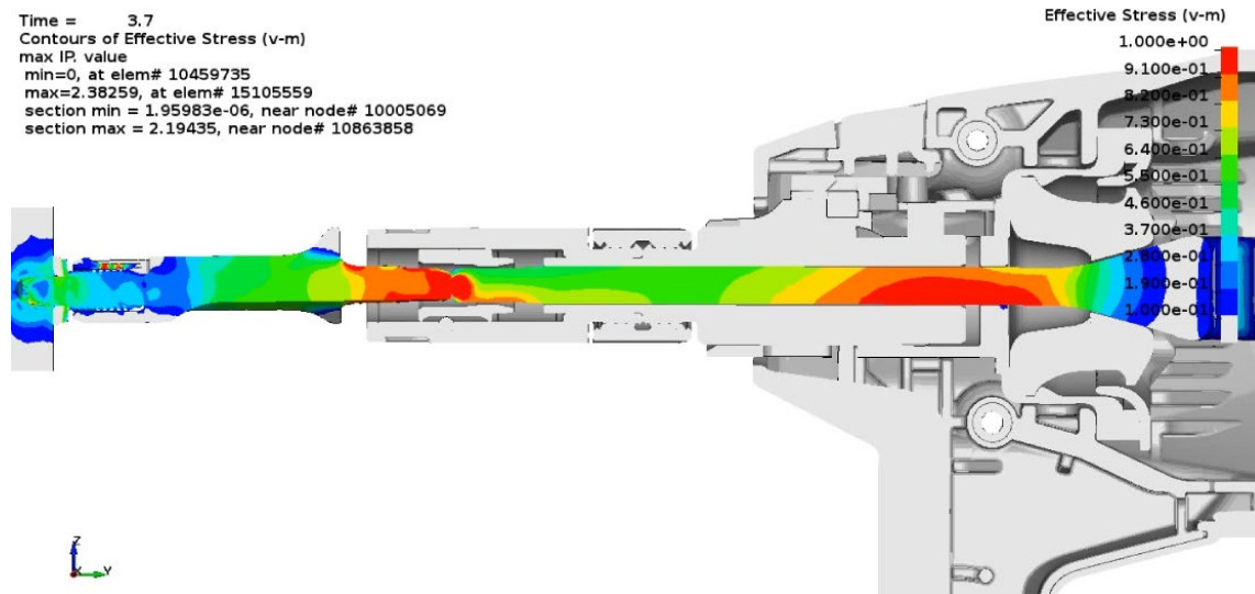
Stress distribution in a cross- section of a direct fastening tool
