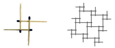
Left: basic reciprocal frame structure, right: example of a composite reciprocal frame structure.
