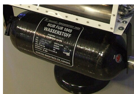
H2 tank made of fiber laminate
