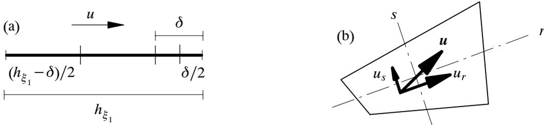
Fig. 8.2: (a) Shishkin-type mesh creation (1-D); (b) velocity vectors at center (2-D)
