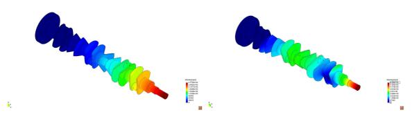
Figure 7.28: Absolute displacement amplitudes of crankshaft at excitation frequency 26 Hz (left) and 162 Hz (right).
