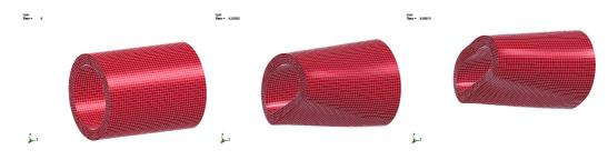
Figure 1.3: Deformation of a steel tube in a drop test, see OLOVSSON AND SIMONSSON (2006).
