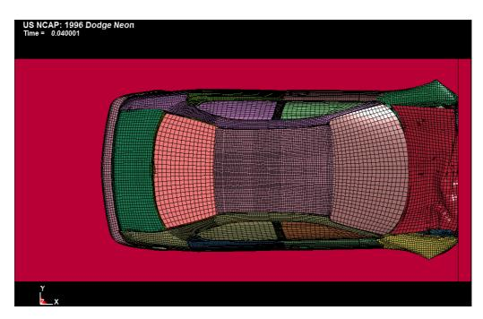
Figure 1.4: Deformed shape of a Neon 1996 model after 40 ms for the initial velocity 15.6 m/s.
